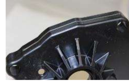
Conformal dispensing on 3D substrates (i.e. out of injection moulding)
