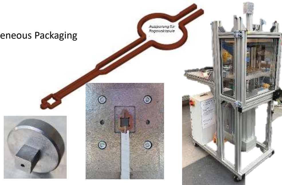
Induction coil with pressure tooling (left), experimental test rig for sinter processes (right)
