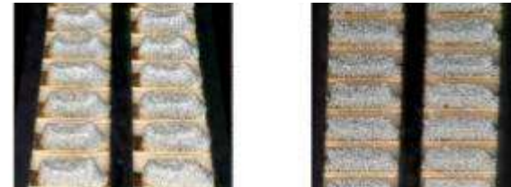
Figure 6 Optical inspection of the solder joint soldered with conventional flux solder paste (left picture) and a sample soldered with fluxless solder paste (right picture) (magnification: 60x)
